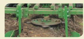
**High Quality Boron Steel Reversible Blades**These self sharpening blades cut the stubbles below ground level
