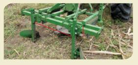
Adjustable Tines with Small Ridger Suitable for different sugar cane planting systems
