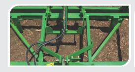
Large V-shape channel 25 cm V-shape channel helps in creating upto 20 cm high basin.
