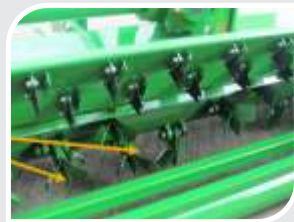
Rotor Mounted Blades With electronic balanced rotor shaft, less vibration and increased life of bearing and belt
